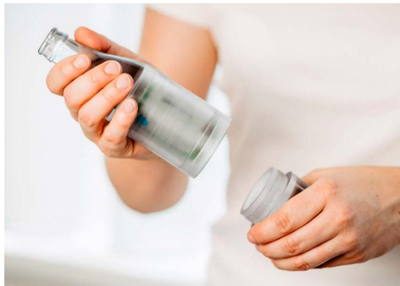
The sensor inserted in the dummy registers potential danger points for the glass container in the line.
