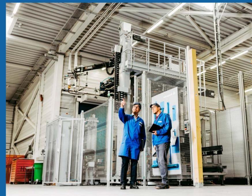
RFID technology for pallets is already in use at our Pöchlarn, Straža, Nemšová and Kyjov plants. The solution records data for both incoming and outgoing pallets. Going forward, it will be possible to divert individual pallets to external depalletising zones according to defined criteria, and to ensure the traceability of the pallets with the articles.
